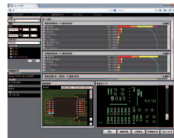
• Analysis function Shows real faults and false alarms in Pareto chart
